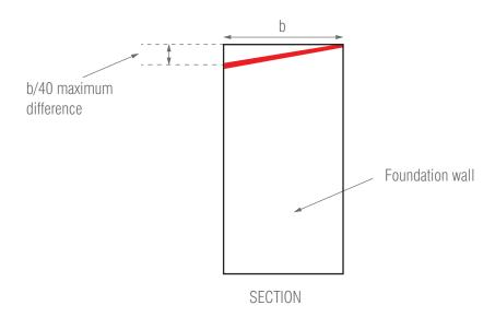
Note: Steel work support frames are to be level and flat to the structural timber designer's specification. Packing on steel work relies on solid packs making leveling of the superstructure more difficult if the support steels are not flat. Concrete and masonry support walls can be leveled by suitable mortar bedding. Depth of bedding to be to the project engineers specification. See Part 2 of this guidance
