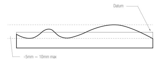
Flatness of the surface by which a structure is supported, for example a sole plate on a transfer slab, should be controlled such that the variation is not greater than:
