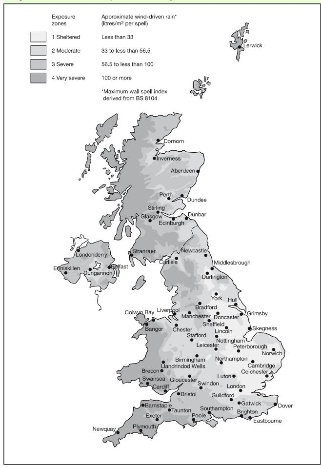
Table 4 Maximum recommended exposure zones for insulated masonry walls
